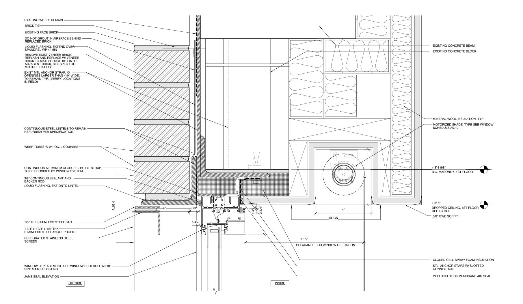
SECTION A WINDOW TYPE 12 TYPICAL - EXISTING LINTELS
